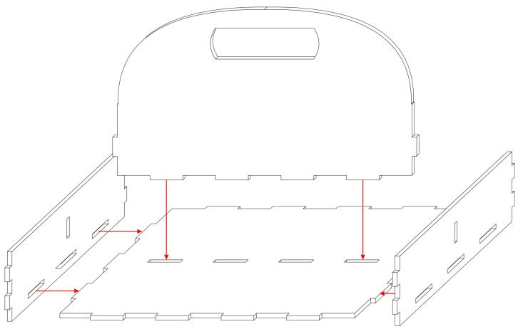
Start the bottom tray by gluing the divider/handle part first. Follow with the side elements. Clamp and leave to dry.
