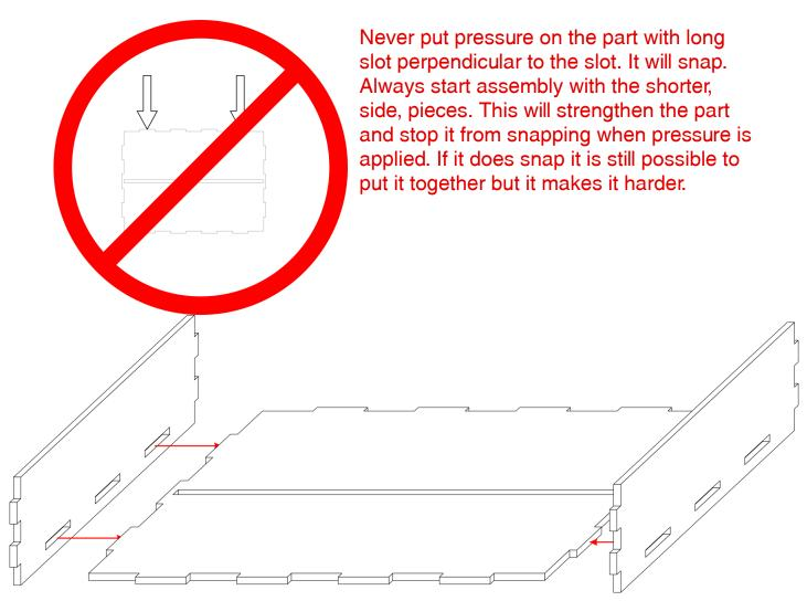
Start assembly of removable tray by gluing the shorter sides first. Clamp and leave to dry. The slots may be tight fitting, use file/sand paper to clean them up and ease assembly. Use plenty of wood glue.
